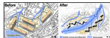
Left: Without wind corridor Right: With wind corridor
